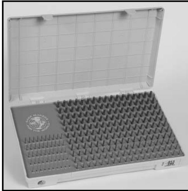
Offers the same “features” as our Class Z pin gages, but with 0.00004” tolerance limits and 0.00002” roundness limits. The pins are perfect for critical inspection needs, or when you want to maximize your GO/ NOGO tolerance limits. They’re also a great way to calibrate measuring equipment, micrometers, and calipers.
