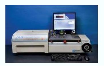
With instrument uncertainty to 2 millionths of an inch (50 nanometers), the Labmaster Universal (LM U306270) is suitable for virtually all Internal (ID) and external (OD) measuring applications. This laser-based universal length measuring system (ULM) has been developed by Pratt & Whitney for gage calibration laboratories that need to precisely measure length, outside diameter, inside diameter, pitch diameter, lead, major/minor diameter, taper, linear displacement, and thickness.
